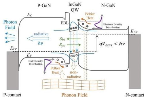
**Figure 3.** Forward biased nitride LED showing the carrier injection and recombination for  $qV < hv$ . Note that the electron and hole high energy thermal tails provide the “missing energy” ( $hv - qV$ ).
